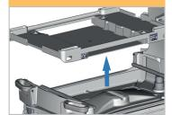
Fit the bed support and push it over the T-bars.
