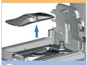
Insert the small cover for the warm air duct.
